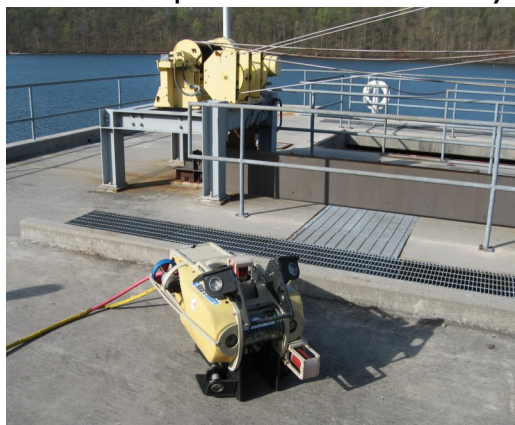
Inspection Vehicle with Sonar and Additional Lighting 3-D Sonar Point Data from Intake at Bifurcation
